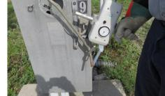
Force gauge dynamometer was connected to handle of MOAB
